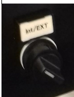
Selector Int/EXT For connection remote controls
