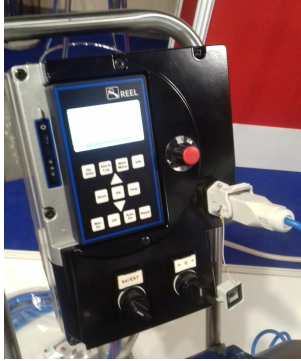
Potenzimeter graduated and counted from 1 to 10 available on a board of inverter
