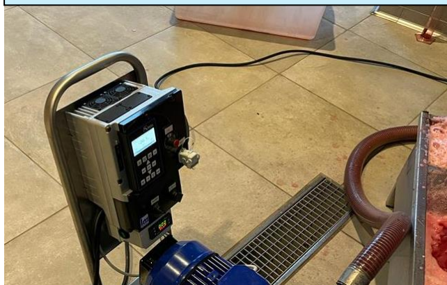
Application example Mounted timer on board pump with INVERTER
